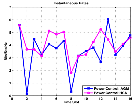
Fig. 2. The instantaneous rate of a user over a block of time slots in power control schemes
