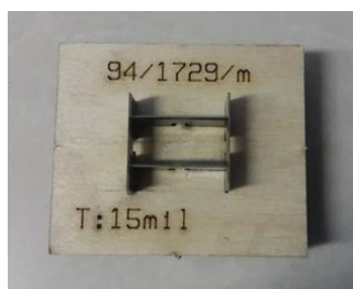
Fig. 2. Schematic of the die cut mold (10.16×22.86mm 2 ).
