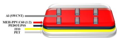
Figure 1. The structure of the fabricated solar cells.
