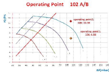
Figure 7. Two points of compressor operating points
