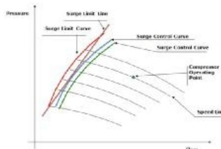
Figure 4. Schematic of surge lines and compressor control
