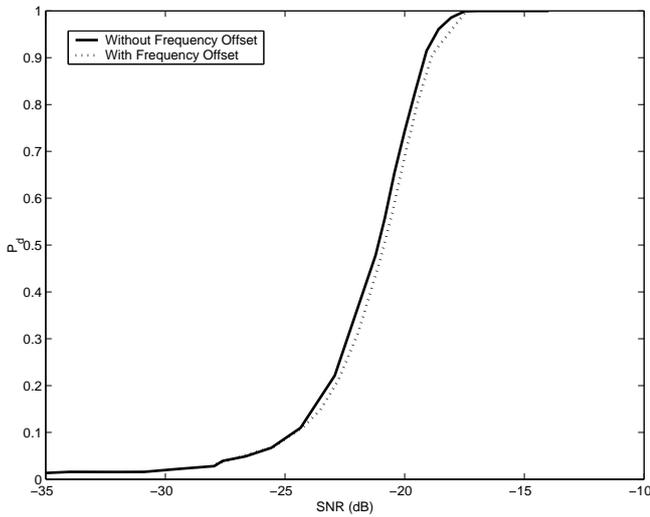
Fig. 3: Probability of detection when the frequency offset of the users are [0.17 0 0.2 0 0.09].
