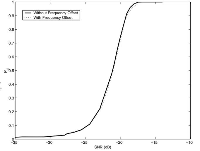
Fig. 2: Probability of detection when the frequency offset of the users are [0.095 0 0.13 0 0.07].
