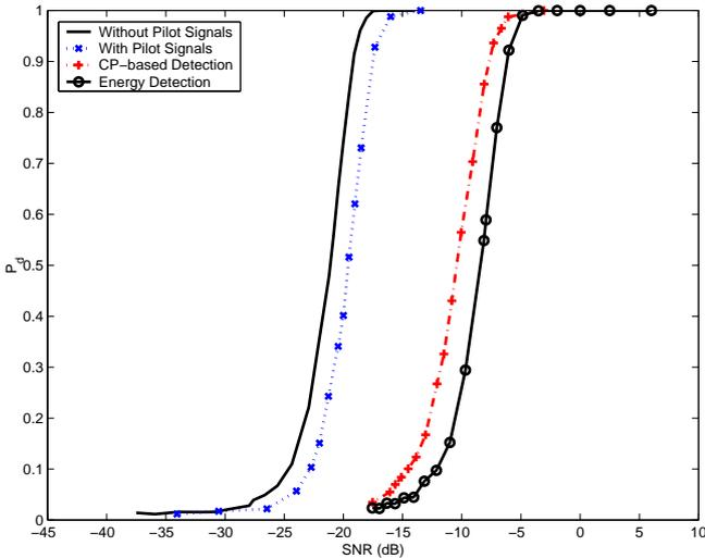
Fig. 1: Comparison of detection performance of our method with and without pilots and that of energy detection and CP-based detection.
