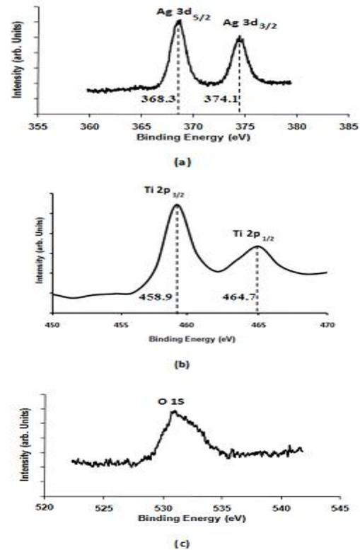
**Figure 3.** XPS spectra of a: Ag (3d), b: Ti(2p) and c: O(1s) core level of the Ag/TiO<sub>2</sub> nanostructure
