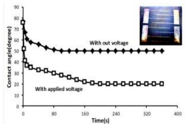
**Figure 6.** Contact angle measurement of distilled water on the Ag/TiO<sub>2</sub> nano-structure under visible light by applying 100V bias voltages on the electrodes.
