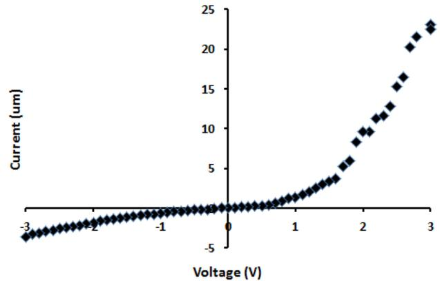
**Figure 9.** Electrical characteristic of the Ag/TiO<sub>2</sub> heterojunction showing the Schottky junction related rectifying behavior.
