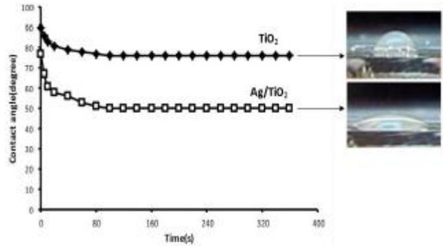
**Figure 5.** Contact angle measurement of distilled water on the TiO<sub>2</sub> and Ag/TiO<sub>2</sub> nanostructures under visible light exposure.
