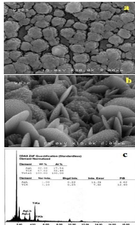
**Figure 1.** SEM images of the prepared TiO<sub>2</sub> nanostructures before (a) and after (b) the formation of Ag nano-particles. Part b demonstrates a magnified view showing the cabbage like TiO<sub>2</sub> coated by Ag nanoparticles. Part c is EDX analysis of the sample showing the presence of Ag nanoparticles on the TiO<sub>2</sub>.
