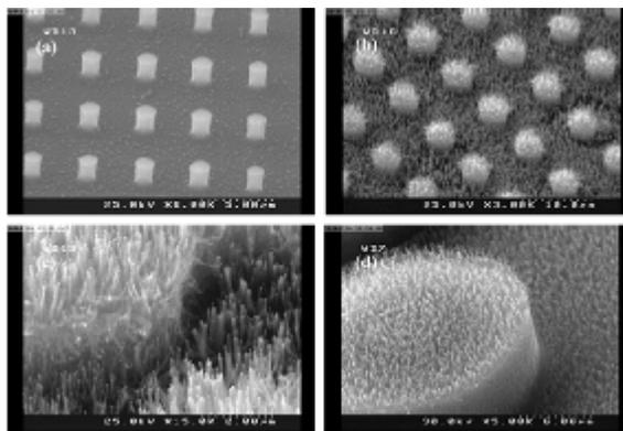
**Fig. 5-** (a) Fabrication of silicon micro cylinders using photolithography and silicon vertical etching process. (b) and (c) the results of coating the sample in part (a) with Ni catalyst using the solution approach and performing CNT growth process on it. (d) For this sample electron beam evaporation system was used for deposition of the Ni catalyst layer. No CNT has grown on the vertical walls.
