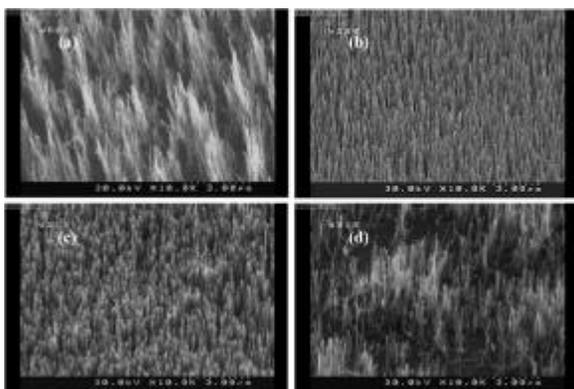
Fig. 3- CNT growth on solution based Ni catalyst coated SiO<sub>2</sub> substrate (a) 35 nm, (b) 53 nm, (c) 98 nm. It can be seen that CNTs are grown uniformly in a wide range on the substrate. (d) CNT growth on solution based Ni catalyst coated Si Substrate.
