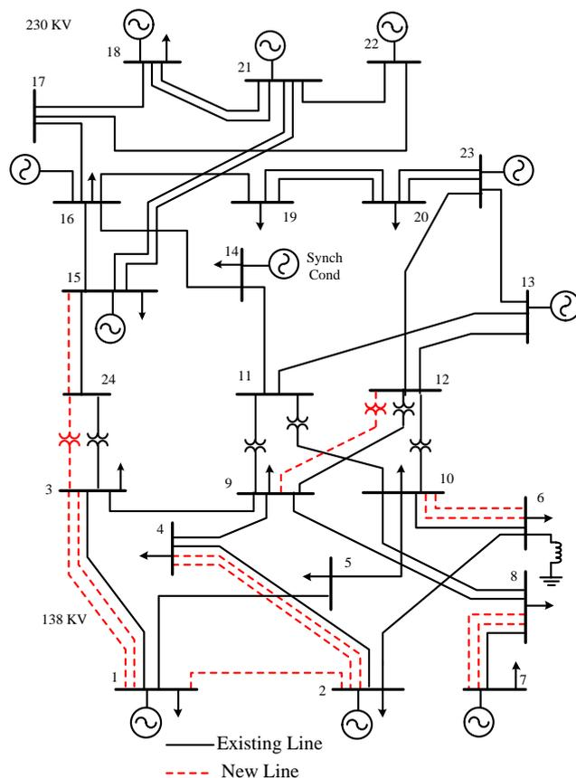
**Fig. 6.** IEEE 24-bus test system after TEP
