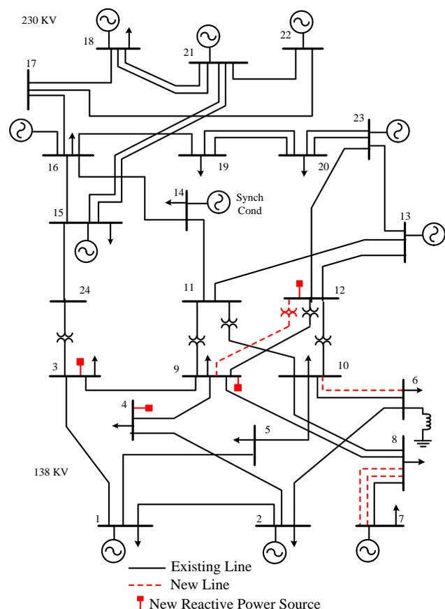
**Fig. 7.** IEEE 24-bus test system after TEP&RPP
