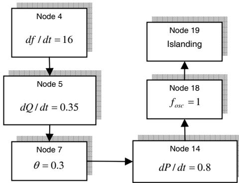
Fig. 13 Operation of the proposed algorithm for loading 1
