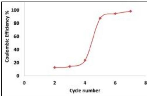
**Figure 5.** The results of coulombic efficiency for the fabricated Lithium ion battery. It can be seen that after 8 cycles of charge and discharge, a coulombic efficiency of 98% is achieved, which is considered as a proper efficiency for lithium ion batteries.
