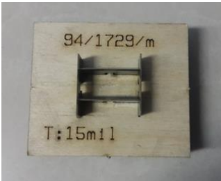
Fig. 2. Schematic of the die cut mold (10.16×22.86mm 2 ).
