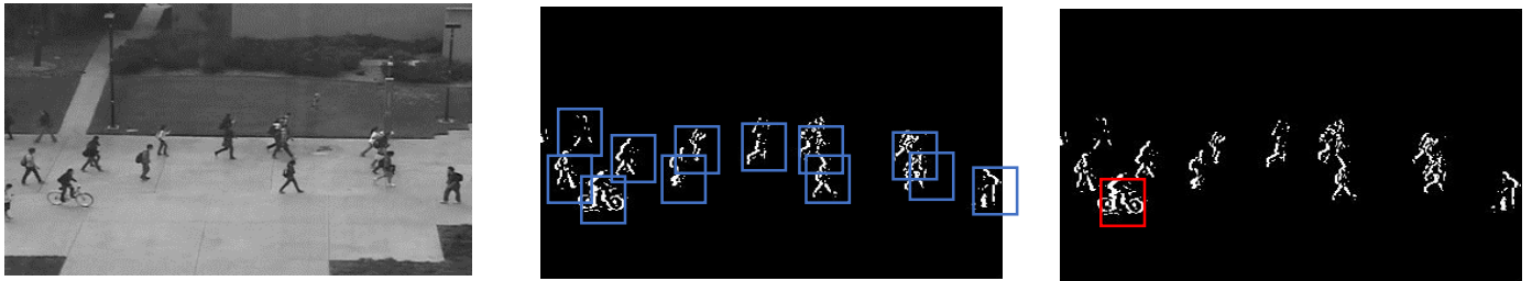
Figure 2. Overall schemes of our method. ( Left ) Original frame ( middle ) Applying a subtraction method for finding those patches which contain an object (here pedestrian) ( right ) that patch which are not fitted to reference model is indicated as anomaly.
