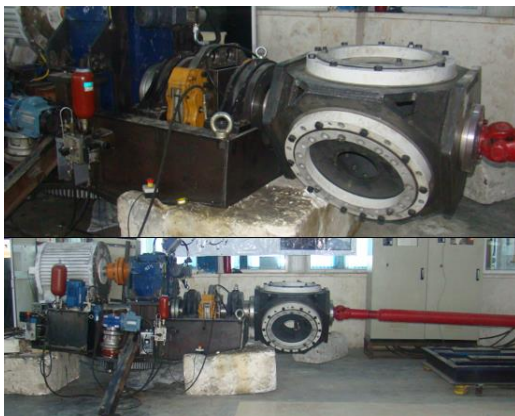
Fig. 22. The practical simulator of 100 KW wind turbine in Sun and Air Research Institute.
