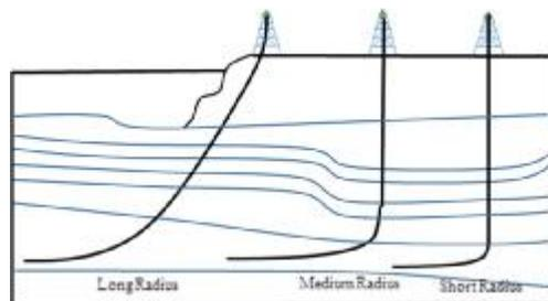
**Figure1.** Several types of directional drilling
