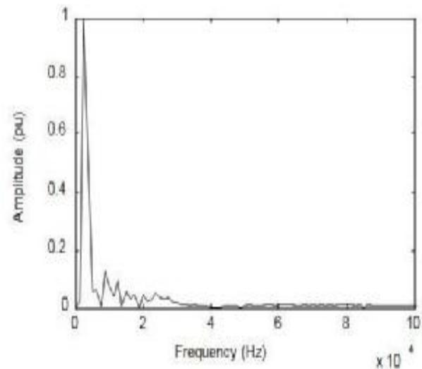
**Figure 3.** S-transform signal energy for fault at bus 814.
