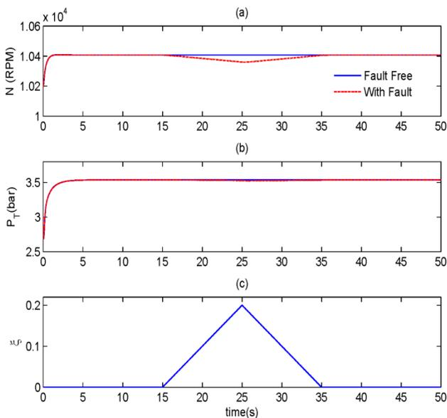
Fig. 2 Output of gas turbine model (fault free and faulty mode); and [(c)]: applied fault  $\xi$
