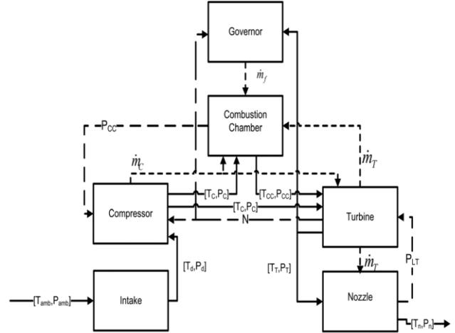
Fig. 1 Information flow diagram in a modular modeling of the gas turbine engine dynamics [31]
