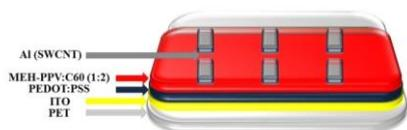
Figure 1. The structure of the fabricated solar cells.
