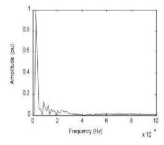
**Figure 3.** S-transform signal energy for fault at bus 814.
