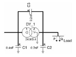
Figure 7. Transformer model for transient study.
