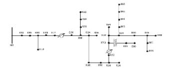
**Figure 8**. IEEE 34-bus distribution test system.
