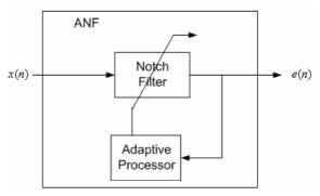
Fig. 1 Adaptive notch filter model
