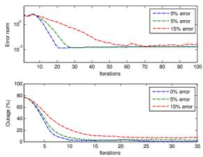
Fig. 12 Convergence behavior of MITDPC algorithm in terms of error norm and outage percentage for gifferent error levels in TPC command
