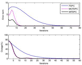
Fig. 8 Error norm and outage percentage for various totally distributed algorithms in static scenario
