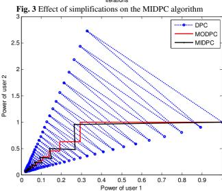
Fig. 4 Power convergence path trajectories for a 2-user system for different distributed algorithms
