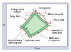
Figure 3. The locus and operating zone of a compressor
