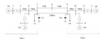
Fig. 2. Two-area four-machine test power system.
