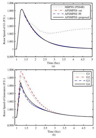
**Fig. 4.** Rotor speed for Case 1: (a) speed of the first Generator (G1) for different types of PSSs and (b) rotor speed of all generators with proposed PSS
