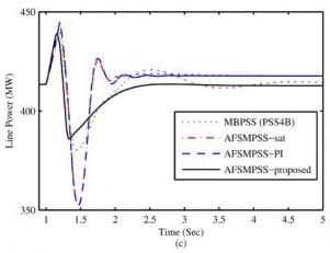
**Fig. 6.** Power System response for Case 2: (a) local mode of oscillations and (b) inter-area mode of oscillations and (c) power transfer from area 1 to area 2
