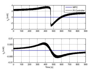
Fig. 10. d-q axis input voltages of Elevation motor
