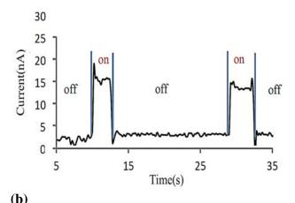
**Figure 3.** (a) Schematic of the ultrasound driven NG and the test setup. (b) The measured short circuit current, when exposed to a couple of on/off cycles of ultrasound wave.
