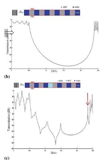
**Figure 4.** (a) Cross section of the investigated NG. (b) Transmission of the perfect 1D PnC, consisting of steel/water slabs with fill fraction of 0.5. The inset displays the unit cell of the simulated perfect PnC, schematically. (c) Transmission of the defected PnC, in which a glass slab is embedded. The inset shows the related unit cell, which consist of a glass-made defect. Horizontal axes are normalized to  $fa/c_T$ .
