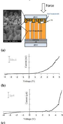
**Figure 2.** (a) Schematic of the fabricated ZnO nanosheet based NG, utilizing nanorod-based top electrode. I-V characteristics of the fabricated NG: (b) without exerting pressure, and (c) with applying external pressure.
