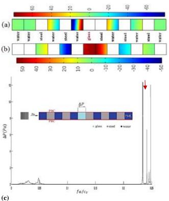
**Figure 5.** (a) Pressure distribution liquid slabs, and (b) solid slabs, in the defected PnC. (c) Pressure difference between two opposite sides of NG versus fa/c<sub>T</sub>, which is maximum at the defect state frequency (red arrow).
