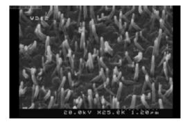
Figure 2. CNTs grown on Si/ITO/Ni surface.
