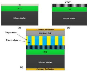
to isolate them from each other. 1M LiPF<sub>6</sub> in (Ethylene carbonate: Dimethyl carbonate (1:1 vol.%)) solution was used as the electrolyte of the battery.
