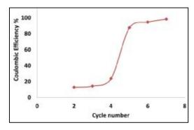
**Figure 5.** The results of coulombic efficiency for the fabricated Lithium ion battery. It can be seen that after 8 cycles of charge and discharge, a columbic efficiency of 98% is achieved, which is considered as a proper efficiency for lithium ion batteries.
