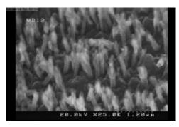
**Figure 3.** CNTs grown on Si/ITO/Ni surface battery test up to 15 cycles.
