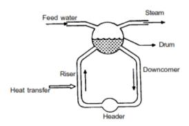
Figure 1. Schematic diagram of drum boiler [14]
