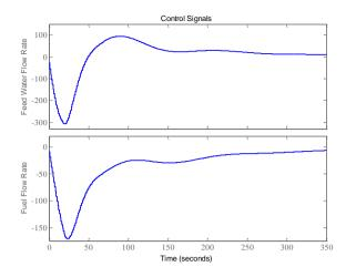
**Figure 6.** Feed water flow and fuel flow rate of boiler under output constraints
