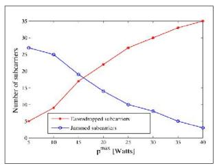
**Fig. 2.** Number of eavesdropped subcarriers and jammed subcarriers versus total transmit power.
