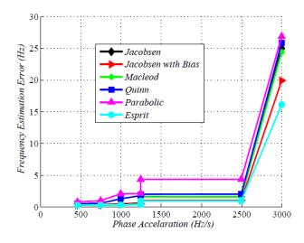
**Fig 4.** Excess Doppler estimation error versus phase acceleration for different estimation algorithms. System parameters: SNR is uniform distributed random variable between -10 dB and 20 dB and sampling frequency rate is 100 Hz.
