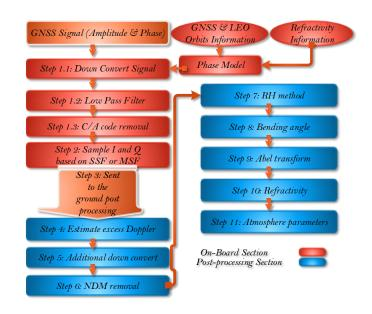
Fig 1. Block diagram of the RO data processing.
