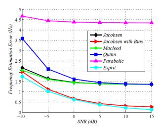
**Fig 3.** Excess Doppler estimation error versus SNR for different estimation algorithms. System parameters: phase acceleration is 1829 Hz/s and sampling frequency rate is 100 Hz.
