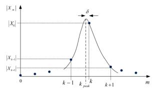
Fig 2. DFT magnitude samples of a spectral tone.
