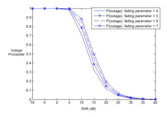
Fig. 3. Outage Probability of Gaussian Point-to-Point channel with different Rayleigh fading parameters
