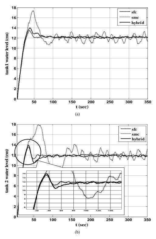
**Figure 6.** Performance of three controllers. The desired value for both tanks is 12 cm, (a) Water level in tank 1 and (b) Water level in tank 2.
