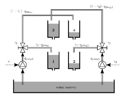
Figure 1. Schematic diagram of QTS.
