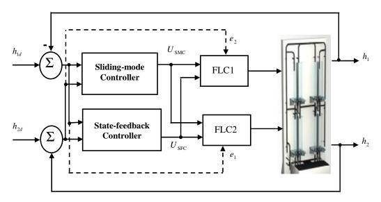
Figure 4. Block diagram of the fuzzy SMC-SFC controller.
