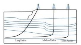
Figure 1. Several types of directional drilling
