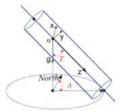
Figure 3. Tilt and azimuth angles [2]
