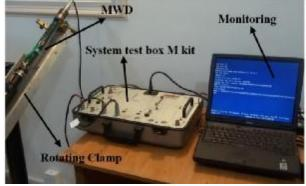
Figure 4. MWD instrument and calibration tools
