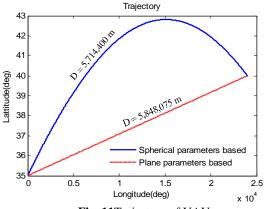
Fig. 11Trajectory of UAV
