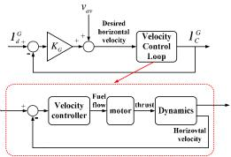
Fig. 8flight time control loop
