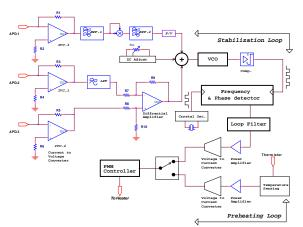
Figure 1. The structure of laser frequency stabilization
