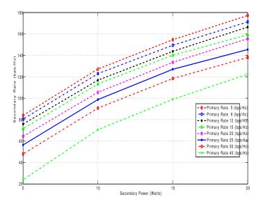
Fig. 2. The effect of changing the transmit power constraint of secondary users on the system throught.
