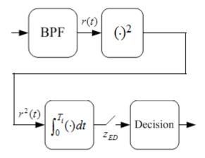
Fig.1. Block diagram of energy detector.
