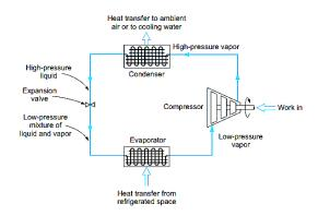
Fig. 1. Schematic diagram of a refrigeration cycle [1].
