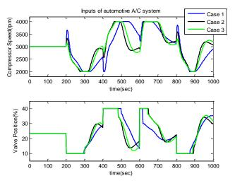
Fig. 3. Inputs of the automotive A/C system via MPC (with two different horizons) and Laguerre based MPC
