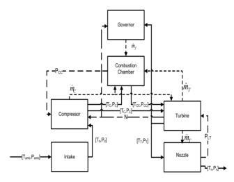
Fig. 1 Information flow diagram in a modular modeling of the gas turbine engine dynamics [31]
