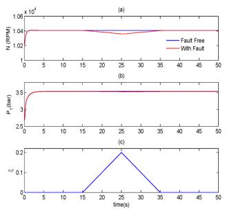
Fig. 2 Output of gas turbine model (fault free and faulty mode); and [(c)]: applied fault  $\boldsymbol{\xi}$
