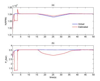
Fig. 3 Estimated states of gas turbine model
