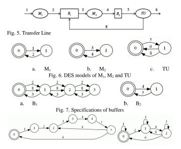
Fig. 8. The supremal relative observable supervisor for transfer line, (*SUP*)
