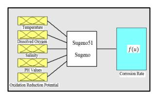
Fig. 4. Input and output variables of ANFIS model.
