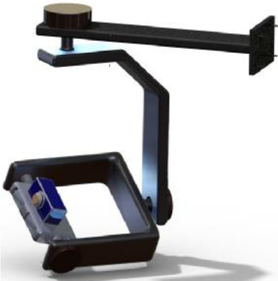
Figure 10.3-axis camera stabilizer conceptual design Specifications of these parts specified in table 2.
