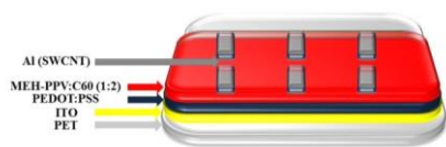
Figure 1. The structure of the fabricated solar cells.
